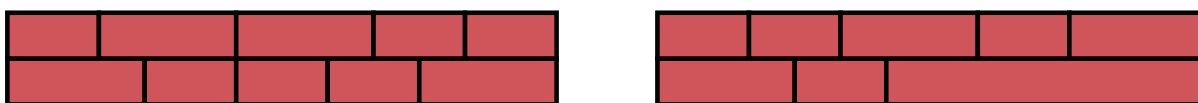
Figure B.1: On the left, we see an unstable wall using the brick types of Sample Input 1. On the right, we see a stable wall using the same brick types. Note that even though only two rows of the wall are shown, it is possible to build an infinitely high wall by repeating these two row configurations.
